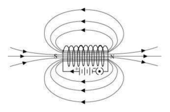
In the above figure, when the north pole of a bar magnet is brought near the end connected to the negative terminal of the battery, the solenoid repels the bar magnet. Since like poles repel each other, the end connected to the negative terminal of the battery behaves as the north pole of the solenoid and the other end behaves as a south pole. Hence, one end of the solenoid behaves as a north pole and the other end behaves as a south pole.
